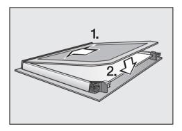
■ Push the inner pane into the plastic strip and place it between the retainers.
